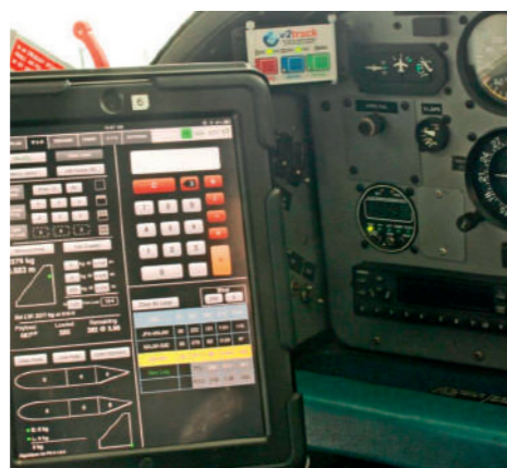
A customer's EFB app linked into v2track via the v2Connect API for data messaging back to base.
